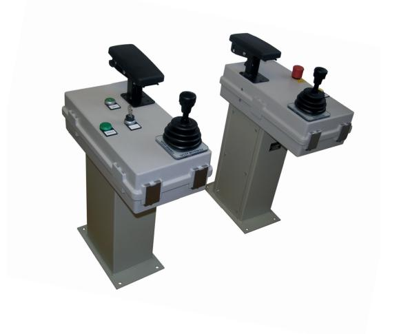
We supply SV0 control station units separately or as a pair, they are mounted directly onto the cabin floor without a bridge. This allows an optimal space adaptation to the operating area. The consoles are available in plastic or metal, the column is made of metal and powdercoated in grey colour.
