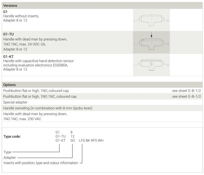
Adapter: 8 = for joystick ST0, CS1-V, VCS0, VNS0 12 = for joystick CS1-E, NNS0, VNS2, NS3, HS2 SO = Special adapter
