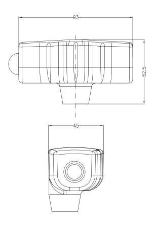
The compact T-handle offers on the left and right side the possibility of fitting one pushbutton with a flat or high cap. The pushbuttons are available as NO or NO/NC. Furthermore, the installation of a capacitive hand detection sensor for fatigue-free work is possible.
